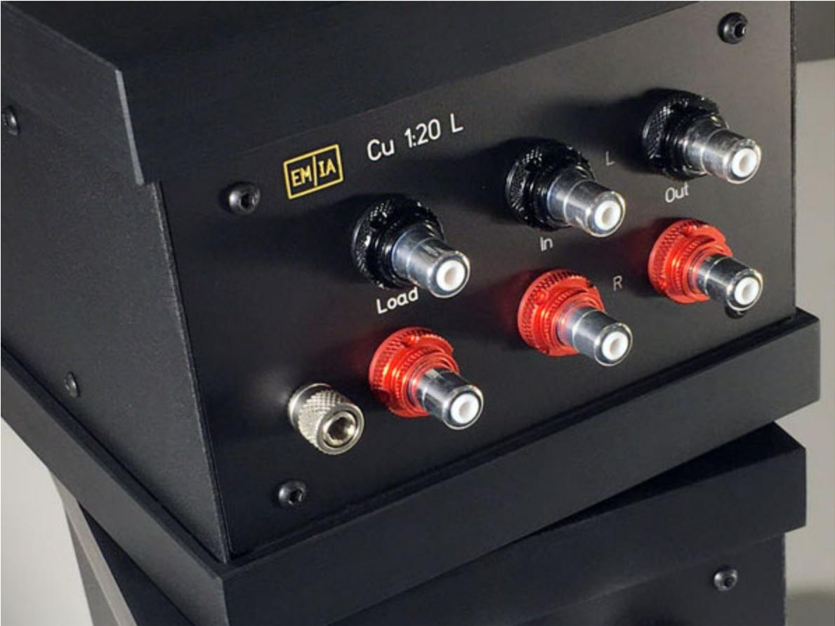
The EMIA moving coil cartridge step up transformers are designed to raise the low voltage output of moving coil phonograph cartridges up to the output level of a typical moving magnet cartridge.
